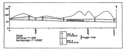
Figure 3.—Cross section of the deposit of sub-bentonite east of Matherville, Wayne County, Miss.
