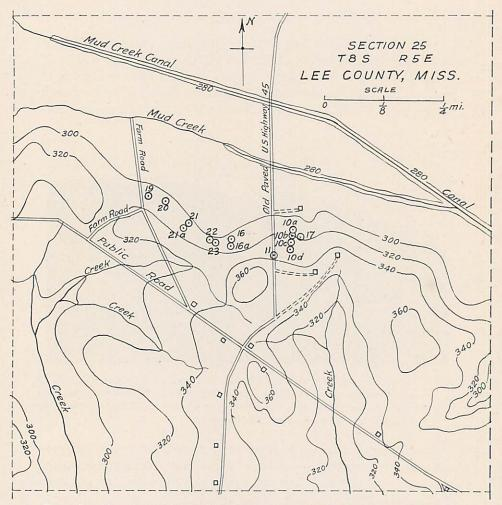
Figure 2.—Map of Mud Creek Bluff at the crossing of old paved U. S. Highway 45 (Sec. 25, T.8 S., R.5 E.) showing the locations from which the samples of chalk were taken.
