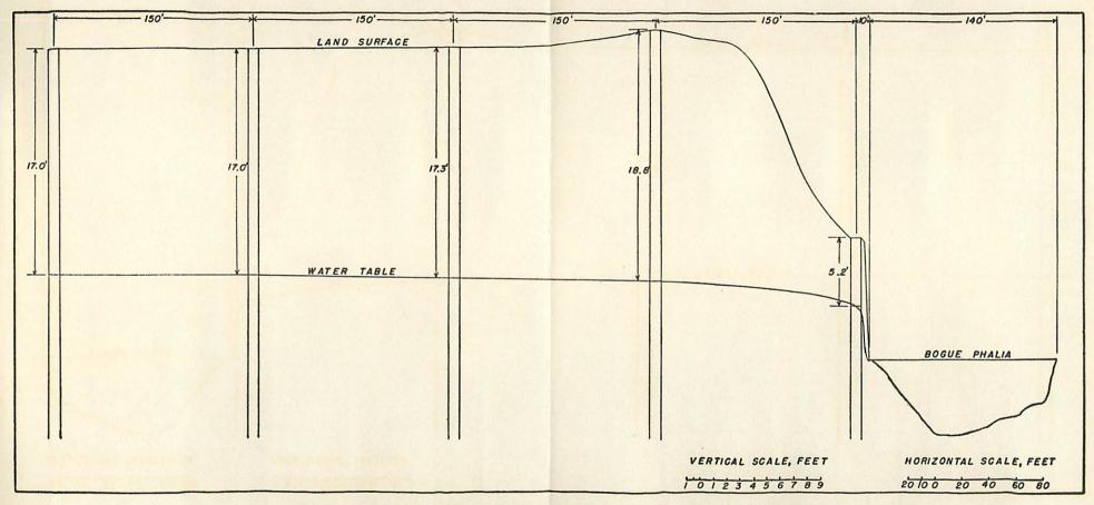
Plate 2 .- Cross-section of Bogue Phalia and test holes at right angle to Bogue Phalia.
