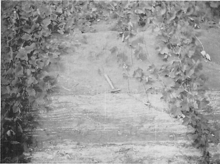
Figure 13. —Lower Ackerman laminated silt and fine sand: Excavation in the east wall of the valley of Little Black Creek, on the north side of U. S. Highway 82, a mile east of Highway 9 in Eupora.
