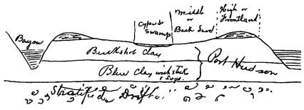
Figure 3.-Section in Mississippi Bottom, Showing Arrangement of Deposits.
