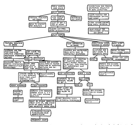
Figure 15.—Flow diagram of preparative procedures and mineralogical-textural analytical techniques.
