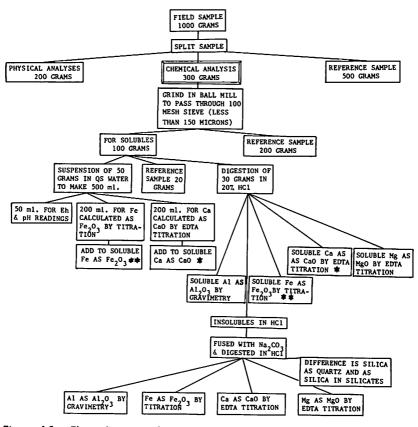
Figure 16.—Flow diagram of preparative procedures and chemical analytical techniques.
