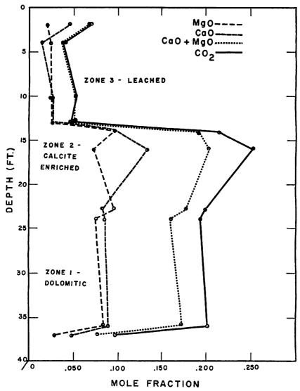
Figure 17.—MgO, CaO, and CO<sub>2</sub> mole fractions in loess from auger hole 3, Warren County, Mississippi, revealing carbonate mineral zones.
