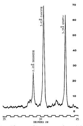
Figure 20.—X-ray diffractogram of loess concretion showing high calcite content due to ground water concentration.
