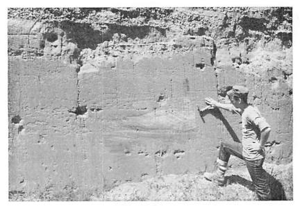
Figure 44.—Cross-bedded "Citronelle" sand and gravel. Surface wash from a 50-foot loess section above obscures the cross-bedding except where it is scraped clean. (Photo taken at sample station 18, Figure 2).
