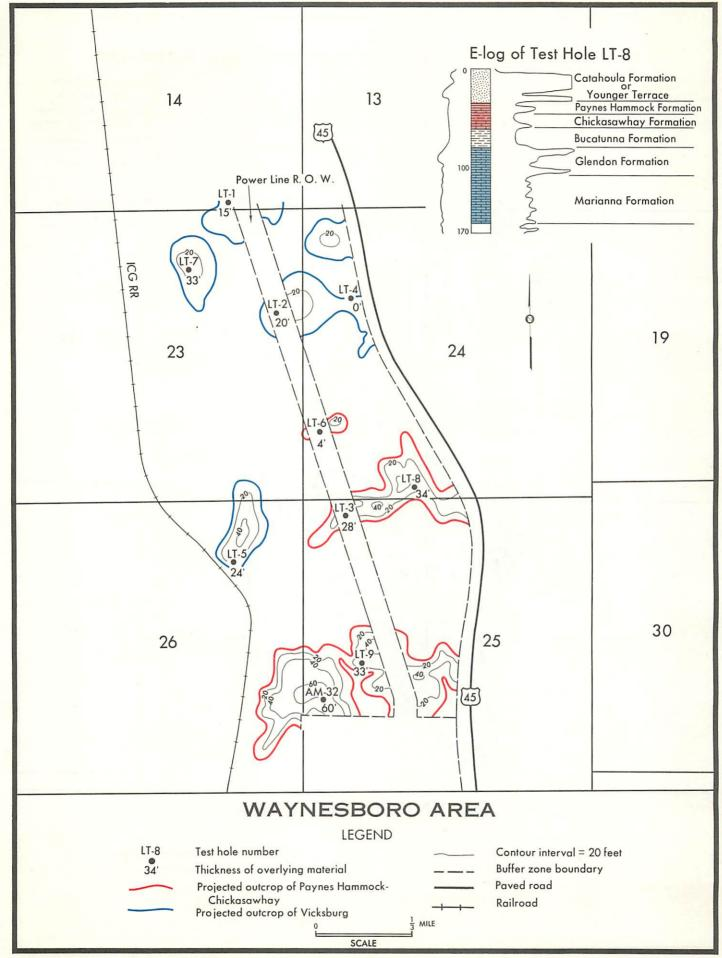
Figure 14 - Projected Outcrop of Limestone and Marl Nearest to the Surface and Isopach of Overlying Material.
