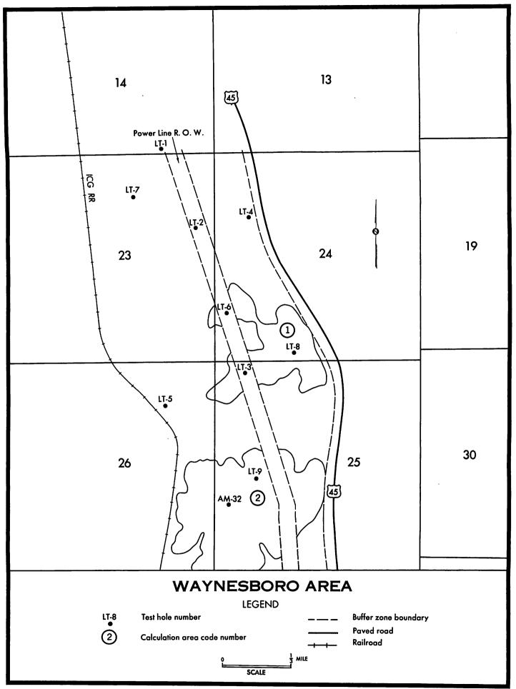
Figure 18 – Calculation Areas for Volume of Limestone and Marl (Chickasawhay)–Calculations based on Estimates of Availability, Quality, Limestone to Overburden Ratio, and Elevation above Natural Drainage.
