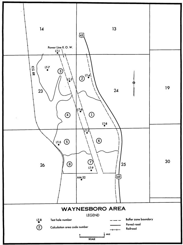
Figure 17 – Calculation Areas for Volume of Limestone and Marl (Vicksburg)–Calculations based on Estimates of Availability, Quality, Elevation above Natural Drainage, and Limestone to Overburden Ratio.
