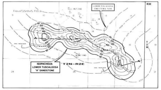
\* Thanksgiving Field is a classic example of a shaleout in three directions against regional dip. The sand pinches out into an abandoned shale-filled channel. This channel plug provides the lateral seal when located on the updip side north of the point-bar sand.
