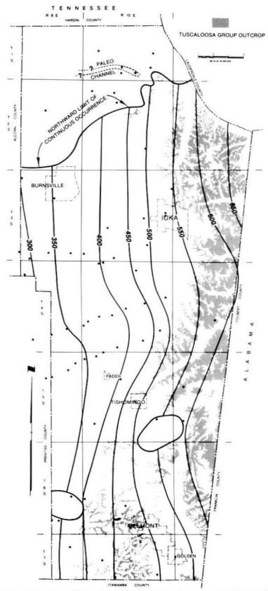
Figure 5. Structure contours, datum top of Tuscaloosa Group, Tishomingo County. Contour interval is 50 feet.
