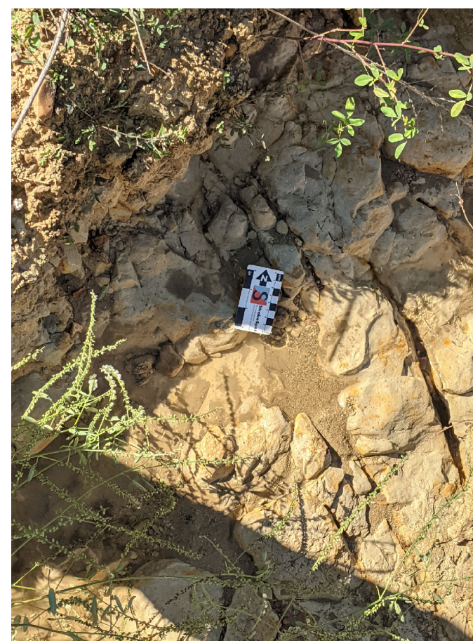
Jointing in weathered Yazoo Clay at the Yazoo City Rubbish Pit in T.11N. R.2W. Section 6, photographed January 5, 2021.
