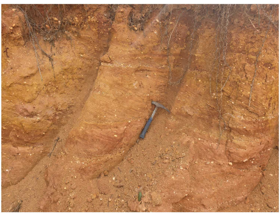
Close-up of cross bedding in limonite stained sand and gravel of the Magee Terrace exposed along the highwall of a surface mine in Section 6, Township 7 North, Range 6 East.
