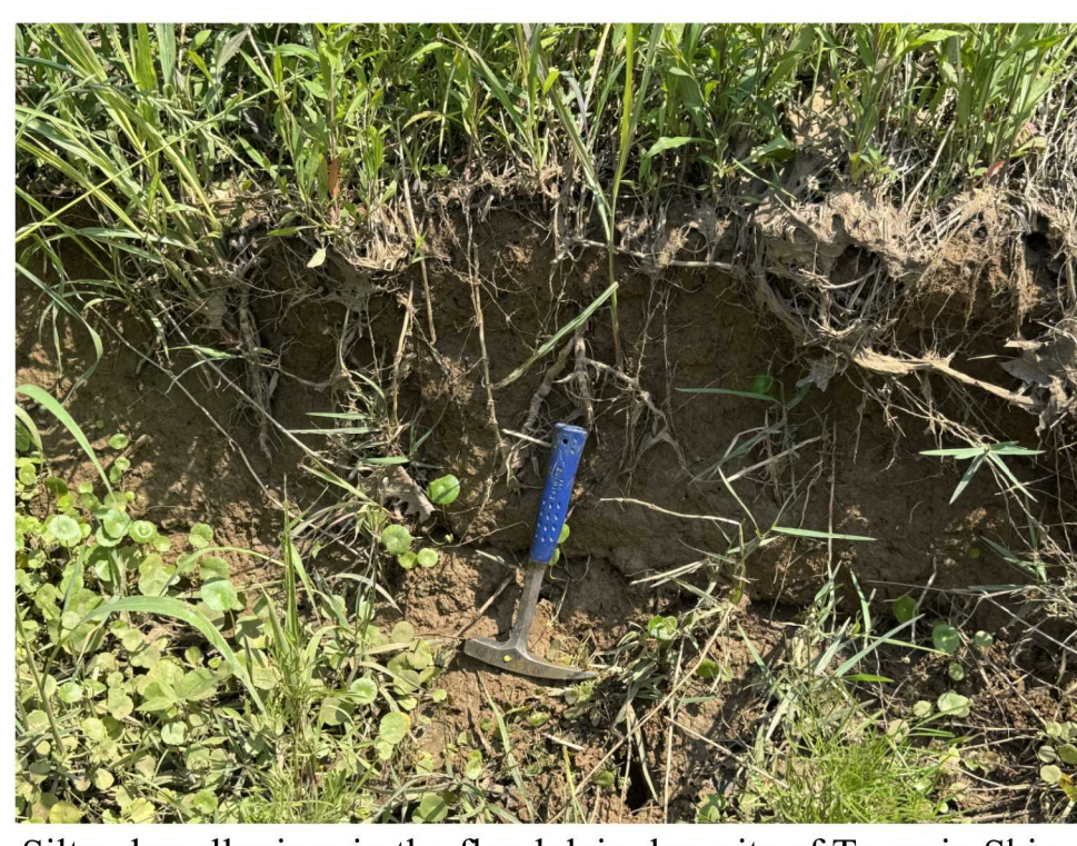
Silty clay alluvium in the floodplain deposits of Terrapin Skin Creek exposed in a slump escarpment beneath vegetation in Section 35, Township 5 North, Range 2 East.
