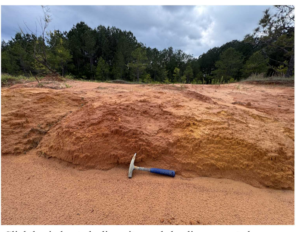
Slightly indurated, limonite and kaolin cemented coarse-grained quartz sands of the Magee Terrace exposed along a road cut in Section 15, Township 4 North, Range 2 East.
