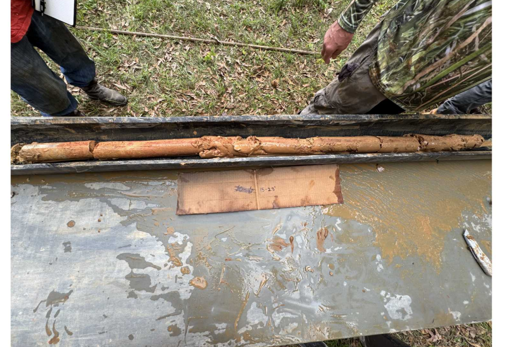
An interval of core penetrating deeply weathered basal clay sands of the lower Forest Hill Formation from a depth interval of 15-23 feet from the MOG Petrified Forest #2 drilled in Section 29, Township 8 North, Range 1 West.
