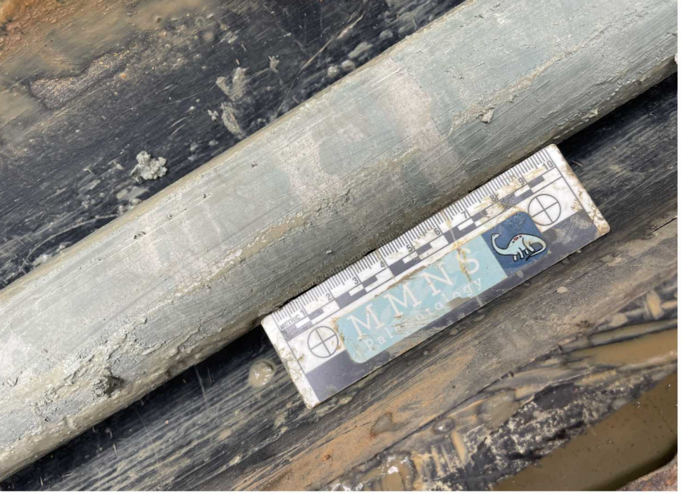
Close up of off-white colored water-lain ash bentonitic clay in interval of core penetrating fresh gray-green colored montmorillonitic clays of the Eocene-Oligocene Yazoo Formation at a depth interval of 63 to 73 feet from the MOG Petrified Forest #2 drilled in Section 20, Township 8 North, Range 1 West.
