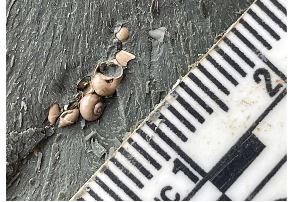
Close up of localized concentration of well-preserved marine gastropods exposed along a parting in an interval of core penetrating fresh gray-green colored montmorillonitic clays of the Eocene-Oligocene Yazoo Formation at a depth interval of 55 feet from the MOG Petrified Forest #2 drilled in Section 20, Township 8 North, Range 1 West.
