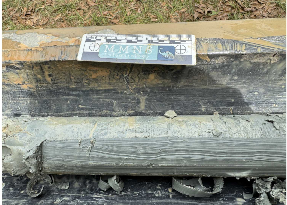
Close up of an interval of core penetrating fresh gray-green colored montmorillonitic bioturbated marine clays of the Yazoo Formation from a depth interval of 43 to 53 feet from the MOG Petrified Forest #2 drilled in Section 20, Township 8 North, Range 1 West.
