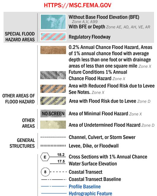
**Base Flood Elevation Line (BFE)**
